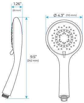
Flow Rate: 2.0 GPM / 7.6 LPM
